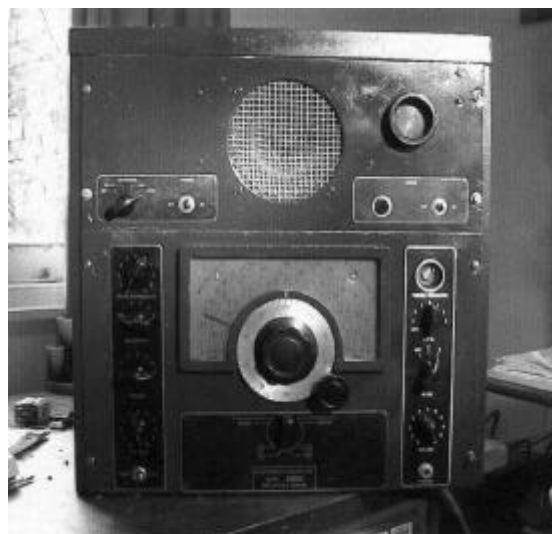
This is Alan Morriss, G4GEN's, VRL, much used recently on the VMARS 80m net. The set itself is in the lower two thirds of the cabinet, with the calibrator, psu and speaker at the top.
