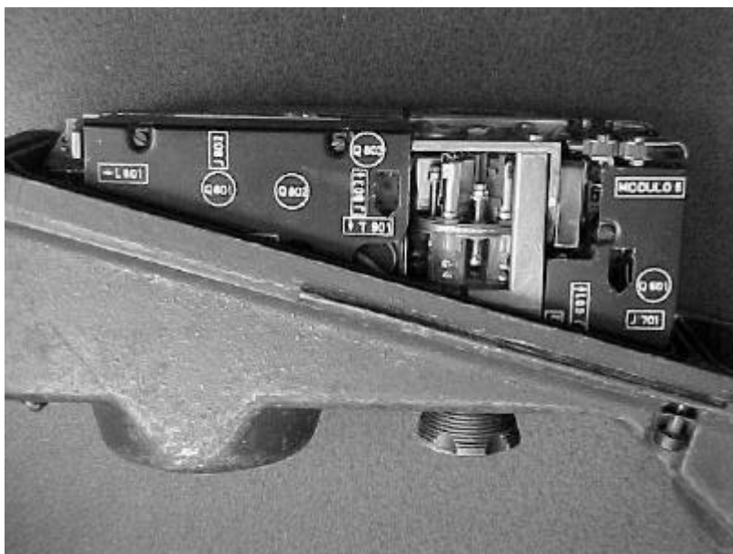
Back case removed showing main chassis and crystal turret
