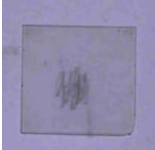
Fig.7. Quartz plate with loading applied.
