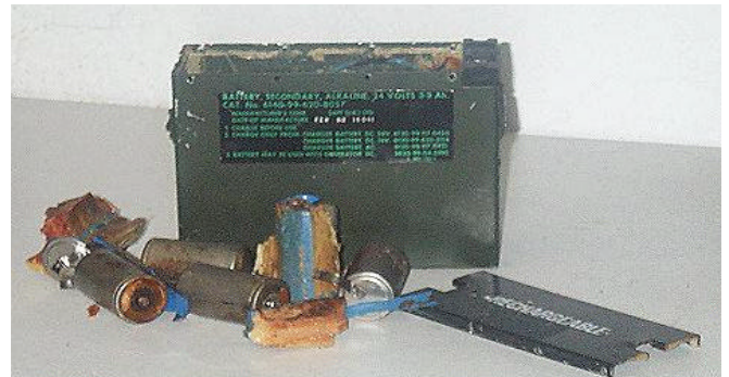
Fig.1 The top layer of cells removed
