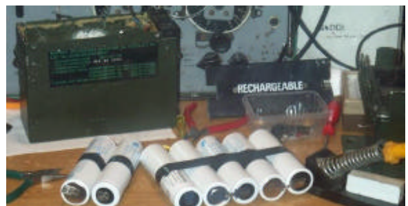
Fig.2 The new cells connected up
