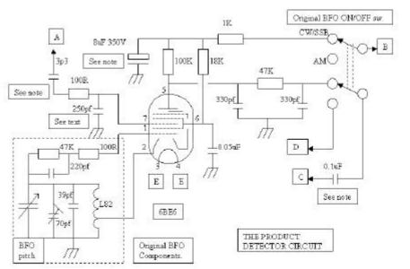
SSB modes. I have checked the level of the IF output signals on my other RA17L's, they are not identical therefore it may be necessary to change the 250pF capacitor to suit.
