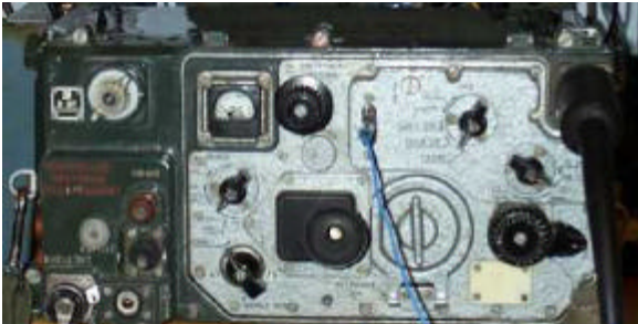
Fig. 2 The lead connected to the OGR socket can be clearly seen
