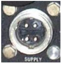
Fig. 3 Supply socket, four male pins, outside diameter 30mm
