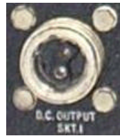
Fig. 4 Output Socket, two female pins, outside diameter 25mm
