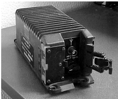
Fig.10 AM-352 RF Amplifier
