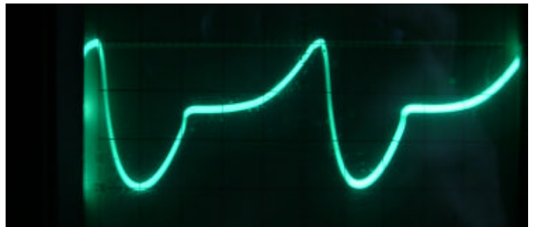
Fig.1: waveform at TR6 base, 37Hz, 15V p-p
