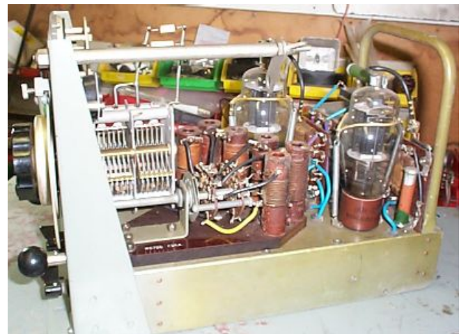
The transmitter drive unit
