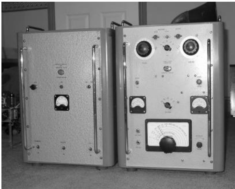
The Labgear LG300— PSU/Modulator on the left hand side, RF unit on the right
