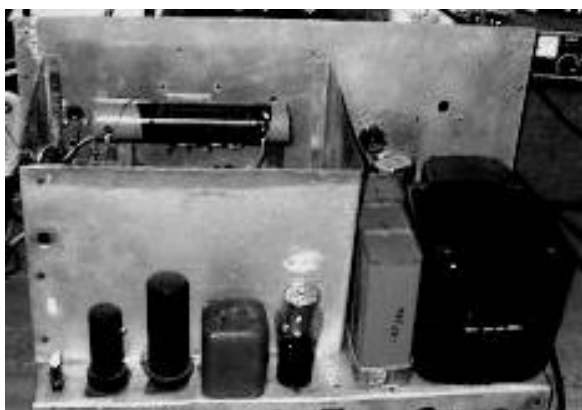
Rear view of RF unit before restoration
