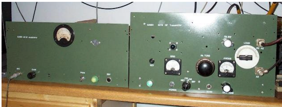
The completed Tx with the Audio Unit on the left and RF unit on the right
