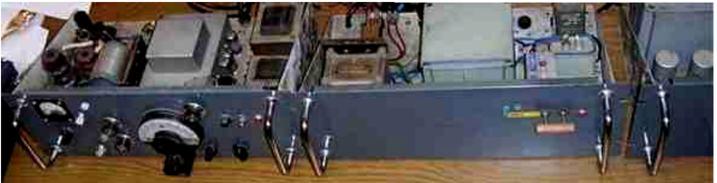
RF deck and power unit as taken out of storage (photo G4NCE)
