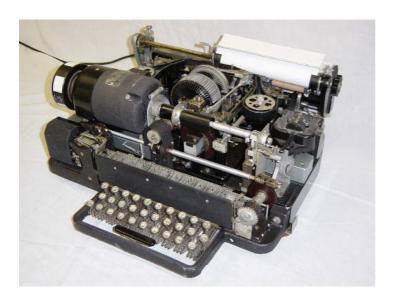
The Creed model 7 page teleprinter, whilst not the first teleprinter to be produced by Creed & Company Limited is, without doubt, the most well known of their machines, and is considered by many to be the teleprinter that helped the Allies to win World War 2. Many thousands of model 7's saw service with the Armed Forces, sending vital messages around the world, and sending top secret messages to and from the code breaking teams at Bletchley Park in Buckinghamshire.
