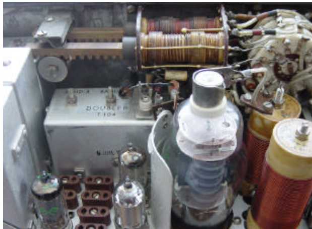
Fig. 1 The 2E22, doubler coils, Band-switch and variable permeability loading coils can be seen.
