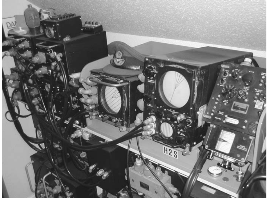
Fig 1 Principal units. Waveform Generator 26, receiver, simulators, Indicator Units 182, 184 and Switch Box 207. Under the table the PSU and Modulator 64
