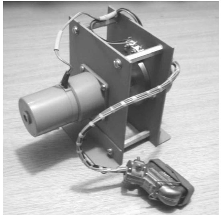
Fig 3 Aerial simulator. This was an early model using a Sin/Cos pot, later replaced with a resolver.
