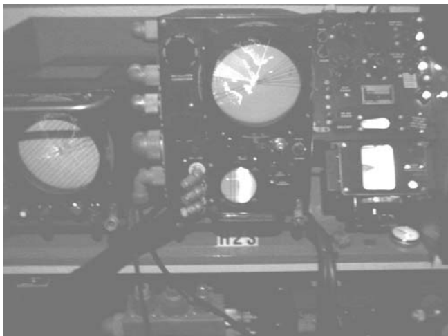
Fig 7 A PPI simulated picture on the Indicator Unit 184. Such is the low light output of the CRT, a VCR517, the picture was taken in almost total darkness.
