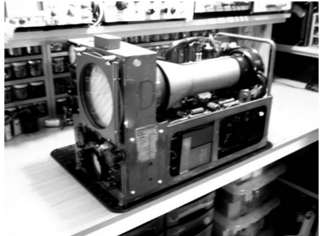
Fig 8 Indicator Unit 162, this was an earlier simpler display than the 184. When a crystal transducer can be made to work, this will form the heart of a Trainer Type 54 simulation.
