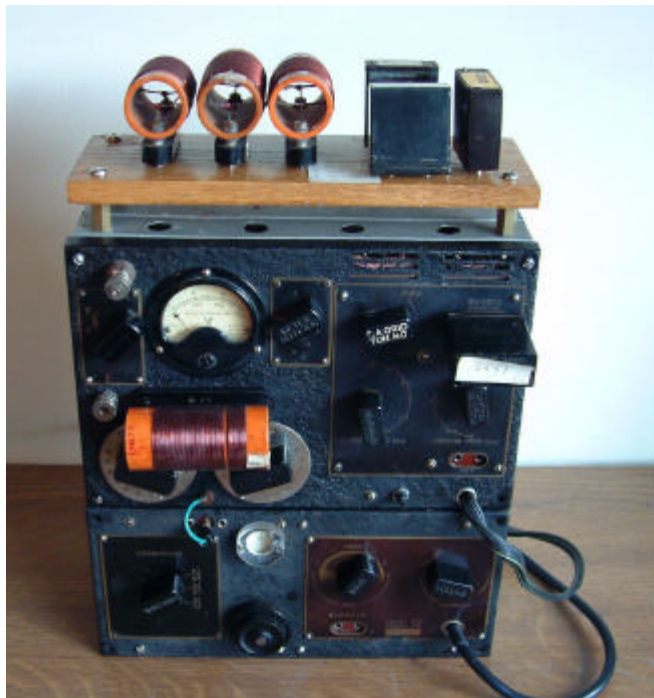
B2 transmitter and receiver. The coil and crystal stowage was added by the previous owner and although not original adds visual interest.
