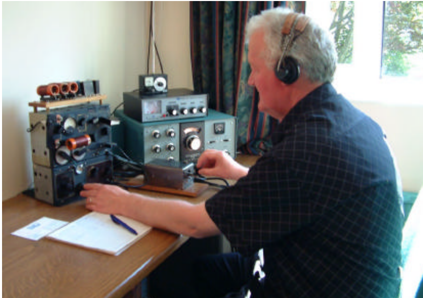
Transmitter and receiver in action with the Japanese Navy key. The Heathkit HW101 is usually used as the receiver but not on this occasion.
