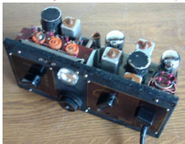
Completed B2 receiver following repairs.
