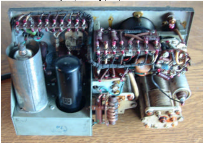
Beautiful simplicity - B2 transmitter with its two valves.
