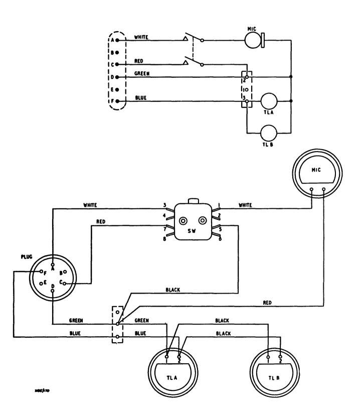
Fig 3005 - Headset microphone, SI type, wiring and circuit diagrams
