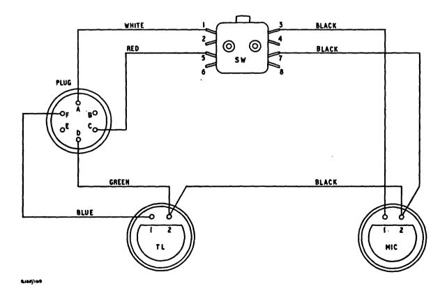
Fig 3004 - Handset, SI type, wiring and circuit diagrams
