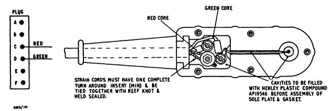
Fig 3006 - SRA13, key, telegraph, assembly detail
