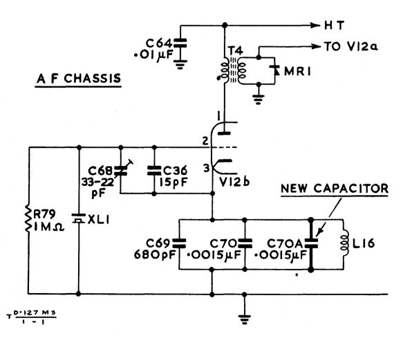
Fig 1 - Calibrator (oscillator section)
