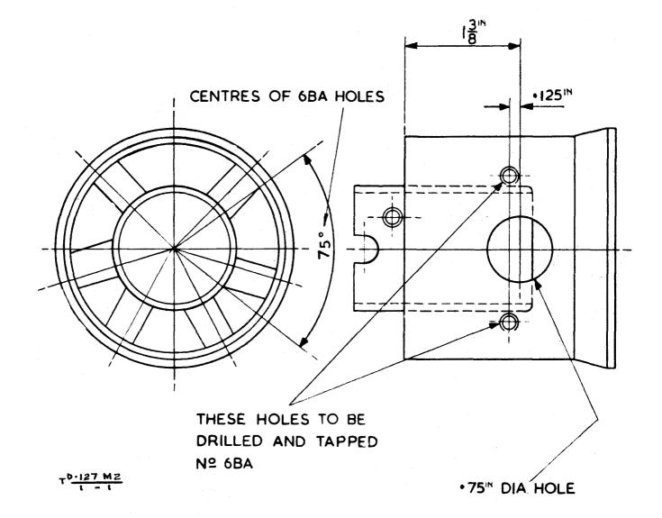
Fig 1 - Drilling details for housing
