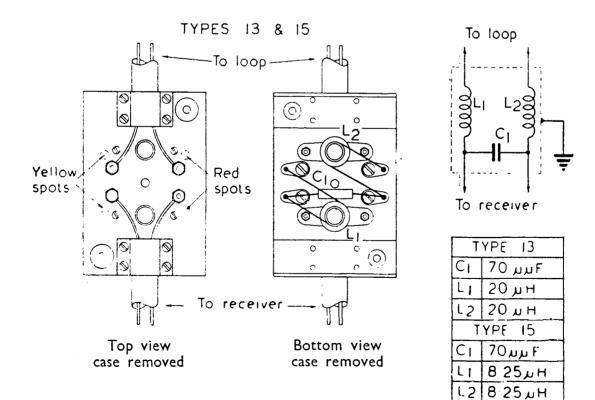
FIG. 24.—THE IMPEDANCE MATCHING UNITS, TYPES 12, 13, AND 15
