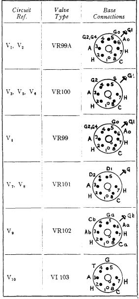
FIG. 20.-VALVE CONNECTIONS
