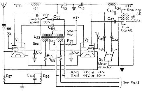
FIG. 11.-L.F. OSCILLATOR SWITCHING CIRCUIT
