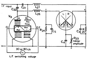
FIG. 13.—SIMPLIFIED VISUAL INDICATOR SWITCHING CIRCUIT
