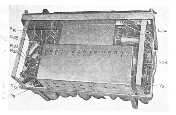
FIG. 16.-R.1155 CHASSIS, UNDERSIDE
