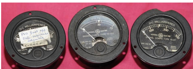
#057 Filament Voltage & PA Current Meters for BC191 / 375
