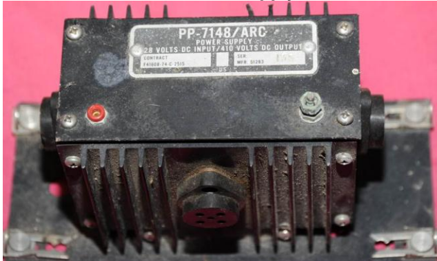
#090 PP-7148/ARC Power Supply 28V in 410V out
