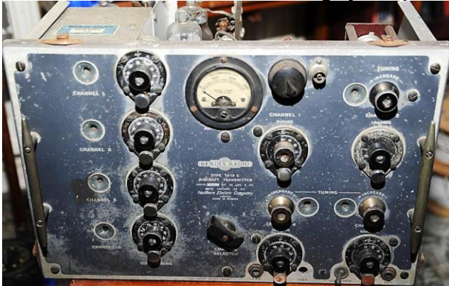
#001 Bendix TA12C Transmitter largely complete
