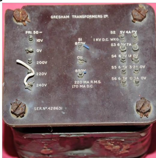
#079 Mains transformer 850 - 0 - 850 V 220 mA RMS
