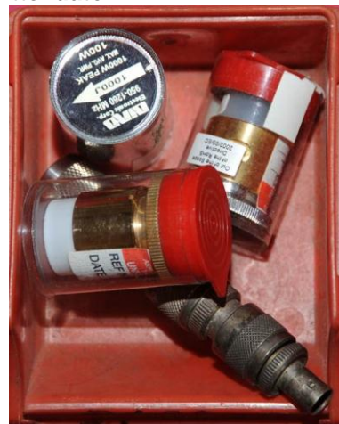
#073 Three Bird Thru-line Wattmeter Elements & Marconi Attenuator
