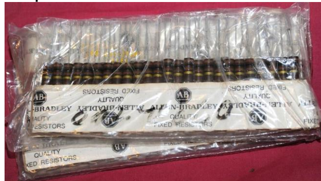
#094 Pack of Resistors 100Ω 2 Watt Carbon Composition
